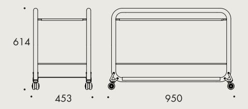
Powder coated frame in Ø32 mm steel tubing. Caster suspension in 2mm powder coated steel sheet. Caster bracket in die-cast zinc, powder-coated. Casters in softened PE, white RAL9010 with black Lammhults logo. Two shelves of 2mm powder coated or stainless steel sheet.
