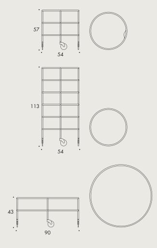
Chicago comes with shelves of frosted glass or laminate, with frame of powder coated or chromium plated steel tubing on casters.
