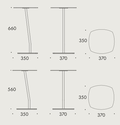
Frame with foot plate of powder coated or chromium plated steel and powder coated pillar of  $\varnothing$ 25 mm steel tubing. Table top of 3 mm powder coated steel sheet. Felt glides.
